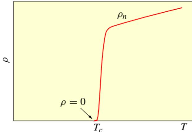
Below the transition temperature  $T_c$ , the resistivity drops to zero.
