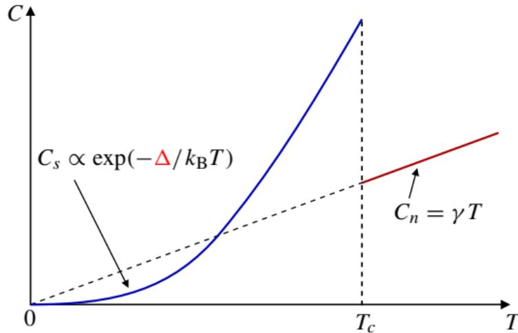
Heat capacity jumps upward on transition to superconducting state. At  $T \ll T_c$  the electronic heat capacity approaches zero exponentially  $\Rightarrow$
