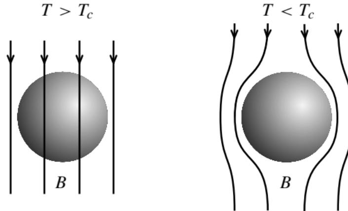
At  $T < T_c$  the **magnetic field is expelled** from the superconductor even if the field was applied before reaching  $T_c$ .
